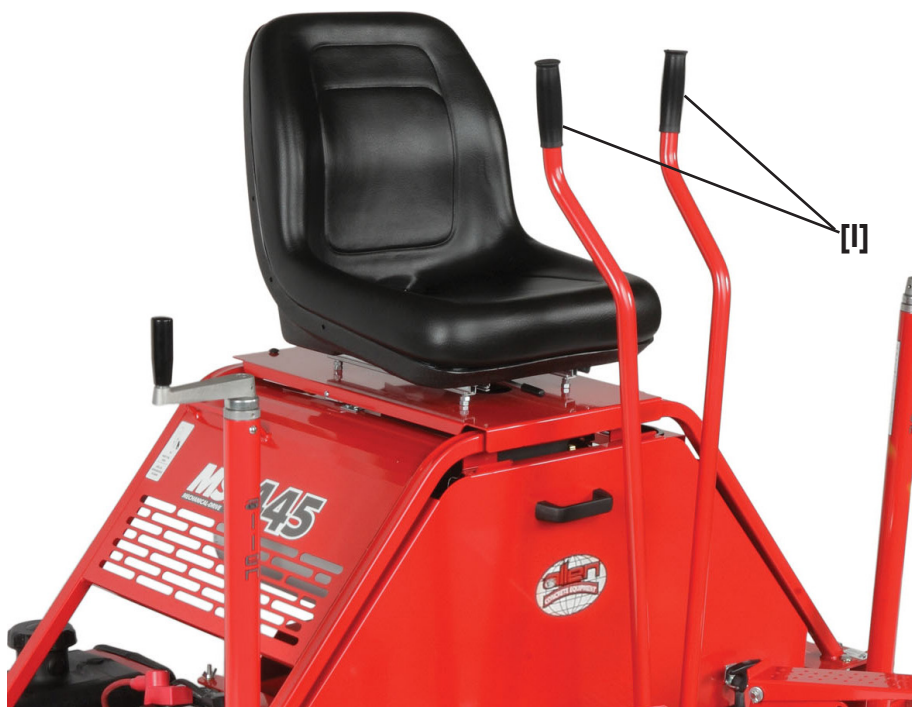
FIGURE 3.7.1 STEERING LEVER LOCATION
