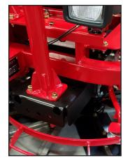
**NOTE**: Utilizing the lifting sling (bridle) and the dolly jacks are intended only for site transportation and the installation of pans and blades. DO NOT use them for regular maintenance without the additional use of jack stands to insure stability of the machine.
