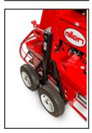
Dolly Jacks are available for HDX riders to make mobilization easier. These tires are foam-filled to help support the added weight of the machine and to help prevent flats. (Comes in set of 2)
