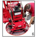
**NOTE**: Utilizing the lifting sling(bridle) and the dolly jacks are intended only for site transportation and the installation of pans and blades. DO NOT use them for regular maintenance without the additional use of jack stands to insure stability of the machine.
